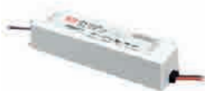
Driver 100a L 190 mm, B 52 mm, H 37 mm, Sec.: 24V, 100 W Schutzart IP67
