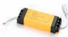
Driver 24i L 135 mm, B 44 mm, H 32 mm, Sec.: 60-82V, 270mA, 24 W
