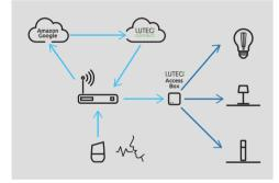
Via Cloud access you can control all the devices in your LUTEC Connect lighting network from anywhere out of home.
