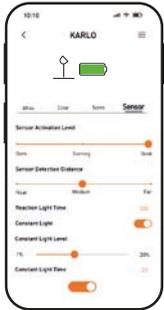
Within the application you can select OFF-AUTO-ON mode. Selecting AUTO mode activates the movement sensor, which enables the light to come on only when someone is passing and increases battery life from a single charge.
