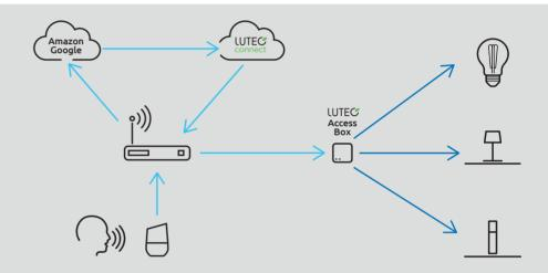
Via Cloud access you can control all the devices in your LUTEC Connect lighting network from anywhere out of home.
