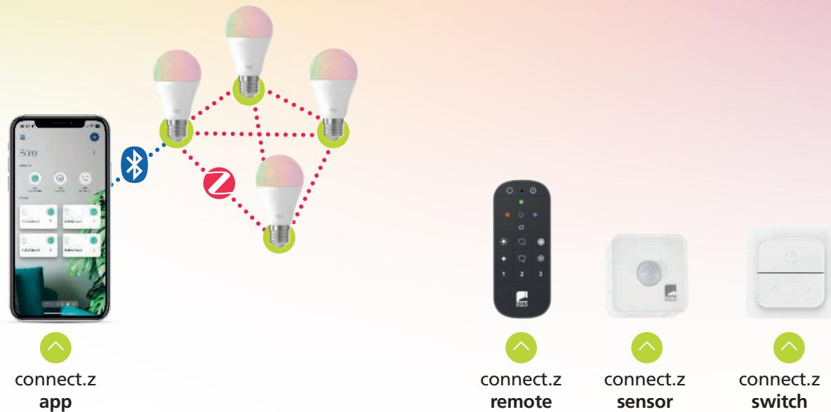
**Connect** our luminaires **directly with Bluetooth and our app - no hub is required**. The luminaires build a stable Zigbee network with each other, so up to 50 luminaires can be controlled using just a smartphone.
